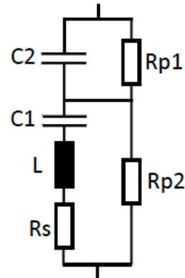
Figure 1. Typical C-type filter design
