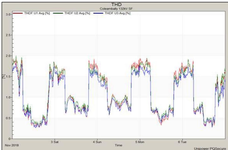
Figure 5. THD measurement plot from TransGrid
