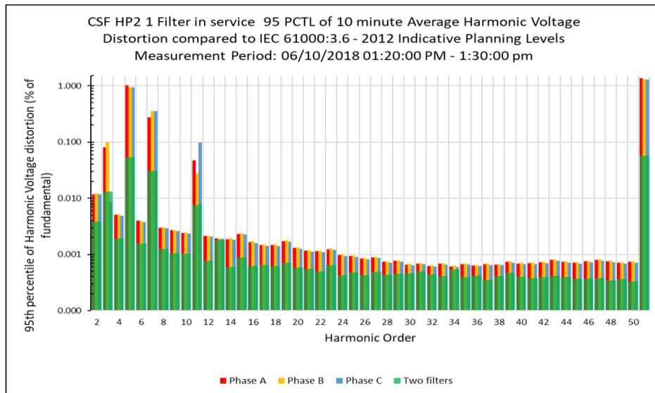
Figure 4. Comparison of measured harmonic emission levels with and without the harmonic filters
