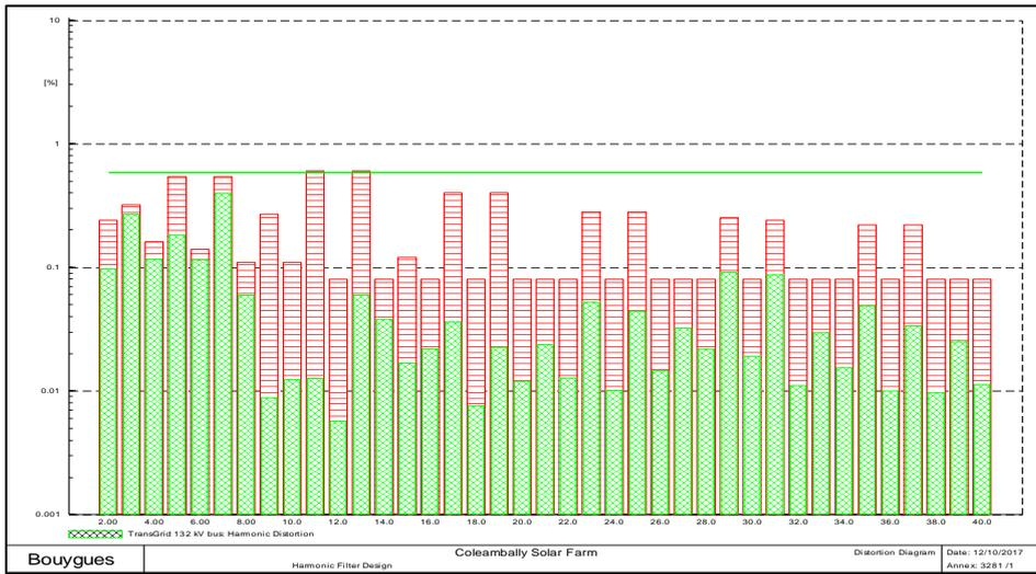
Figure 3. Harmonic distortion diagram
