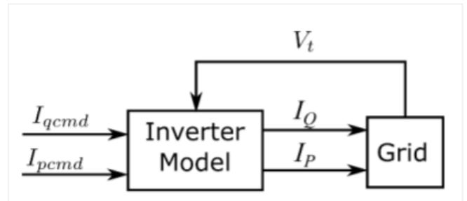
Figure 1: A generic inverter generator model [5]
