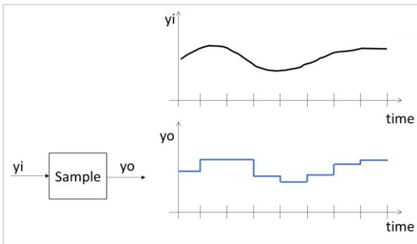
Figure 15: Output of sample and hold block
