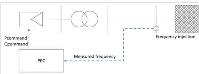
Figure 12: Setup for model simulation of frequency control test
