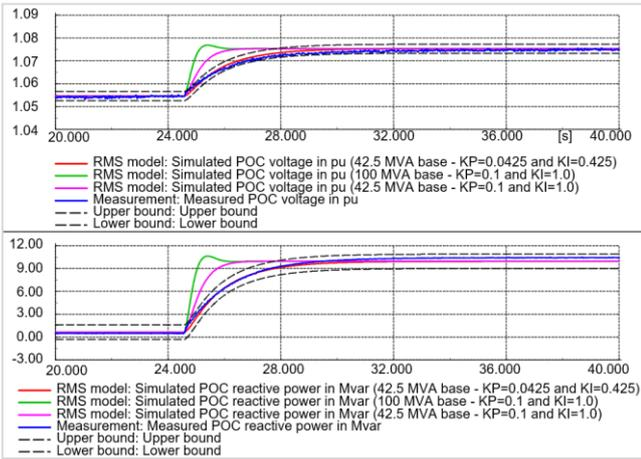
Figure 10: Overlay of voltage and reactive power response to a positive step in power factor setpoint, with different machine base MVA and PPC gain parameters
