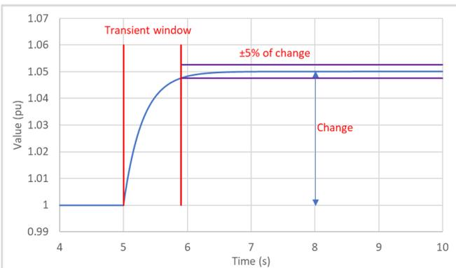
Figure 3: Transient window definition for controlled change
