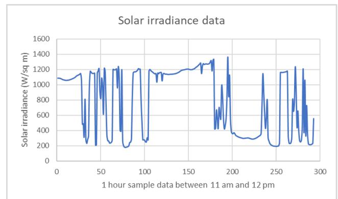
Figure 13: Variation in solar irradiance due to cloud shading
