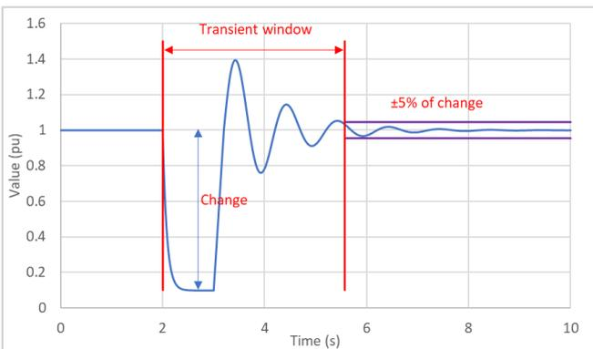
Figure 4: Transient window definition for uncontrolled change
