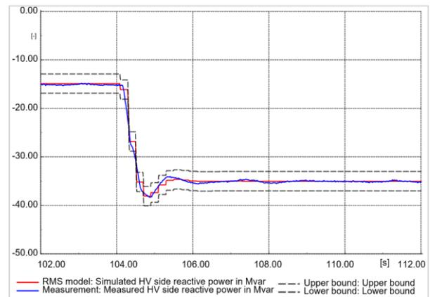
Figure 5: Overlay of  $Q$  response to a negative 20 Mvar step
