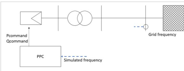
Figure 11: Setup for on-site frequency control test
