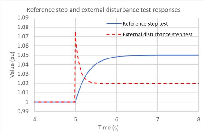
Figure 2: Example of reference step and external disturbance test responses
