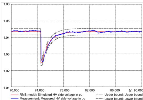
Figure 9: Overlay of  $V$  response to capacitor switching out
