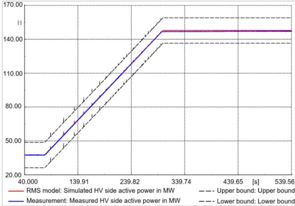
Figure 7: Overlay of  $P$  ramping up response
