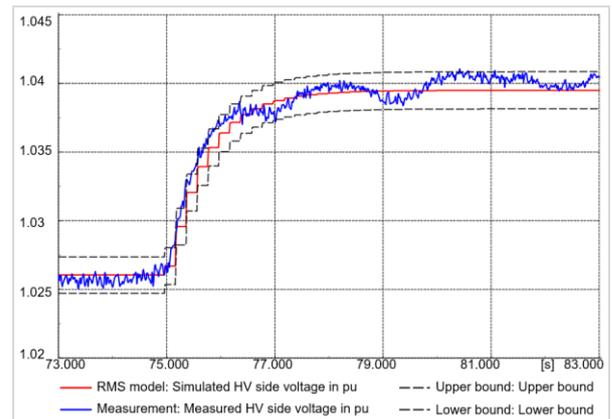
Figure 6: Overlay of  $V$  response to a positive 2.5% voltage step
