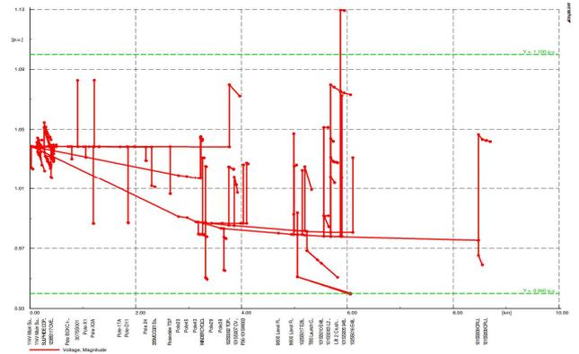
Fig. 3 Existing average loading with existing taps
