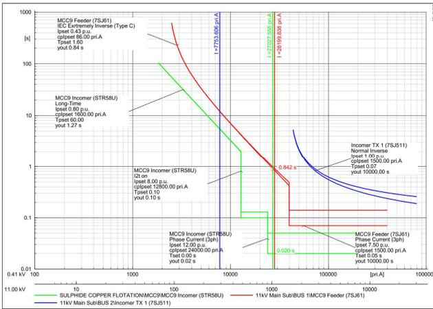
Fig. 2 Protection coordination of upgraded relay
