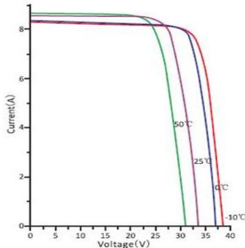
Figure 4 Example of solar panel I-V variation with temperature [10]
