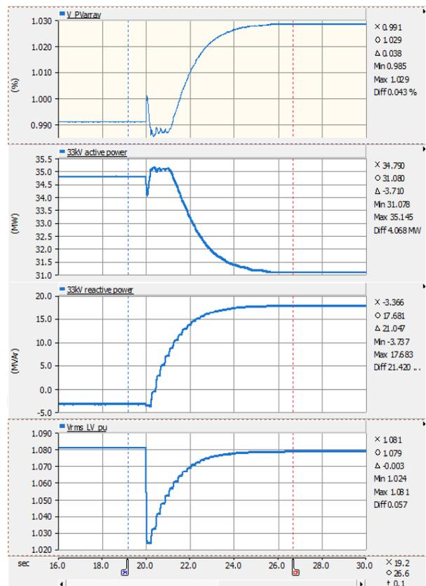
Figure 5 Illustration of active power change for a voltage step. From top to bottom, the graphs are Vdc, MV active power, MV reactive power and Inverter AC voltage
