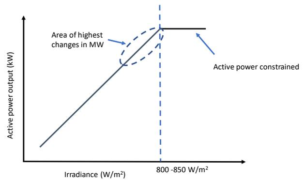
Figure 3 Active power versus irradiance showing region of highest MW change with V<sub>dc</sub> change
