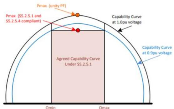
Figure 1 PQ capability curve, to meet continuous uninterrupted operation under S5.2.5.4 [6]
