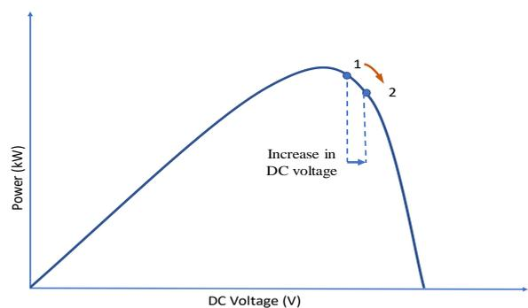
Figure 2 PV array power output versus Vdc
