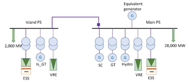
Figure 1: 30 GW power system model used to illustrate primary frequency control co-optimization.
