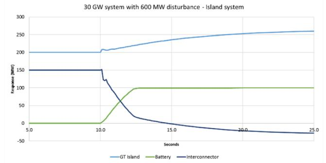
Figure 5: Case 2 Island system response to 600 MW Contingency – Interconnection, Gas and ESS
