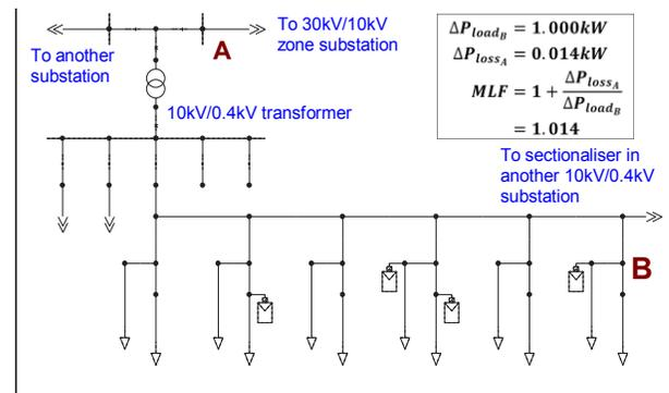
Figure 3. Typical single line diagram of a 0.4kV distribution feeder
