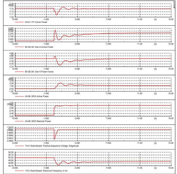
Figure 2. Response of an isolated diesel-PV-BSS hybrid power system to the loss of a diesel generator rated at 2.4MVA and operating pre-fault at 2.0MW
