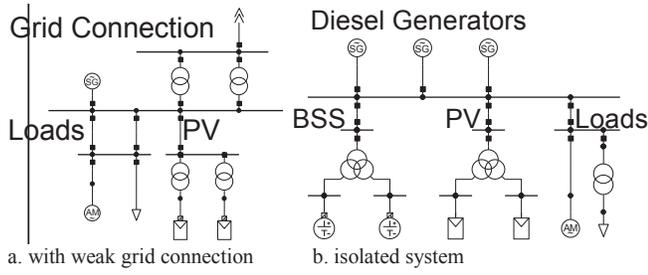
Figure 1. Large-scale solar farm integration at a remote mining site with a weak, single circuit grid connection
