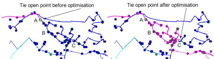
Figure 4. Single line diagram of the network before and after optimisation
