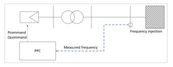
Figure 12: Setup for model simulation of frequency control test
