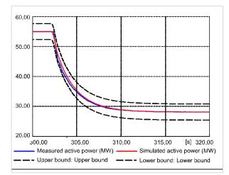
Figure 17: Overlay of simulated response with measured response (sampling rate of 10 ms and PPC cycle of 100 ms)
