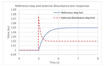
Figure 2: Example of reference step and external disturbance test responses
