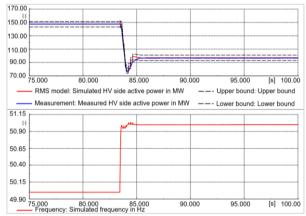
Figure 8: Overlay of P response to positive 1 Hz step
