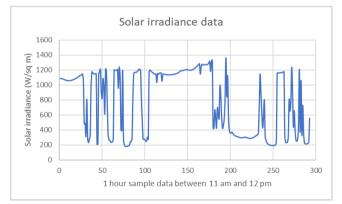
Figure 13: Variation in solar irradiance due to cloud shading
