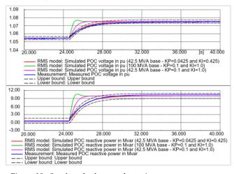
Figure 10: Overlay of voltage and reactive power response to a positive step in power factor setpoint, with different machine base MVA and PPC gain parameters
