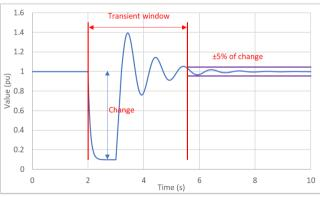
Figure 4: Transient window definition for uncontrolled change
