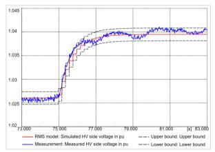
Figure 6: Overlay of V response to a positive 2.5% voltage step
