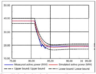
Figure 16: Overlay of simulated response with measured response (sampling rate of 1 s and PPC cycle of 100 ms)
