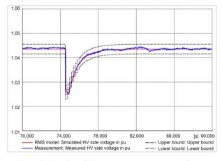
Figure 9: Overlay of V response to capacitor switching out
