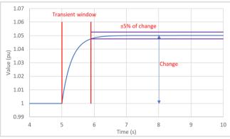
Figure 3: Transient window definition for controlled change
