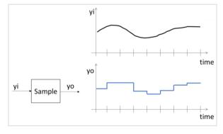
Figure 15: Output of sample and hold block
